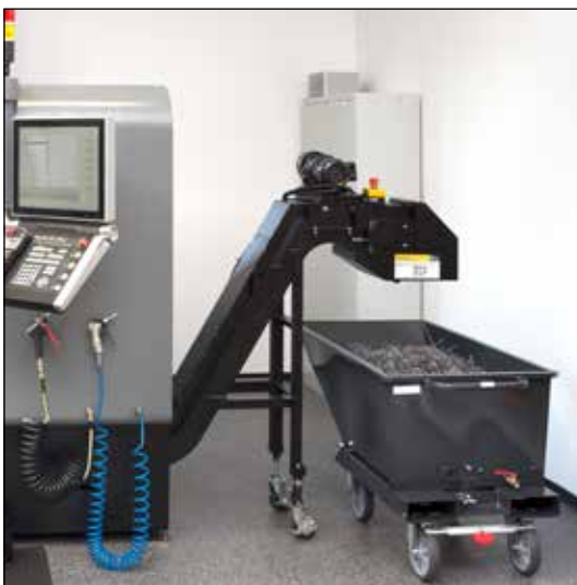
Example of use: Sheet metal dump truck as bin.
