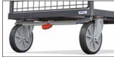
TOTALSTOP - the fetra central brake system With only one foot the rotation of wheels and the swivelling movement of both swivel castors can be securely locked. The brake pedal is always visible to the operator. Standard with TOTALSTOP.
